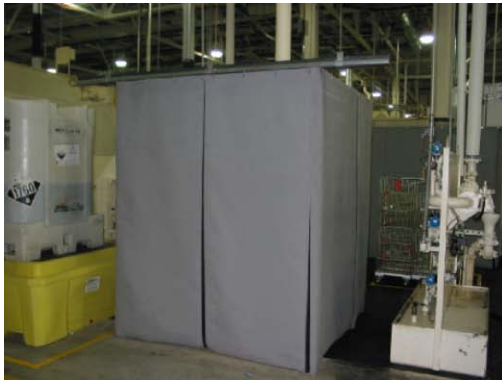
Floor mounted sound curtain enclosure
