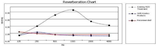
cover the walls, ceiling and floors. With this information we can calculate your room's current reverberation time and use this to determine the amount of acoustical absorption need to be added to the room to bring the reverb time down to acceptable levels. With this data we can propose different products in different quantities at differing price points until we arrive at a solution that meets your budget and acoustical needs.
