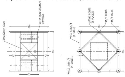
Top view of structural and acoustic panels for entire Sound Enclosure lift-off option.
