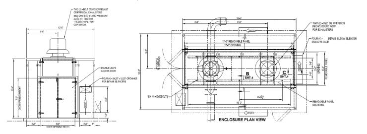
Well Pump Sound Enclosure with access doors, silenced ventilation, and lift-off roof.
