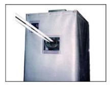
Industrial UN-10 R flexible noise barrier is a 1 lb psf reinforced loaded vinyl barrier used to stop the transmission of noise from one area to another. Typically used as barrier panels in an acoustical enclosure or as the barrier component in conjunction with the FDA Panels for a barrier/absorber composite product. Curtain panels are typically constructed with grommets across the top and vertical edges to suspend and form closures.
