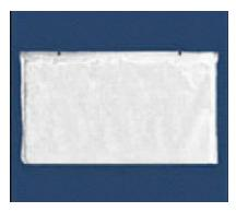
The Industrial **FDA approved baffles** are the ideal solution to reverberation issues in areas where food is present. The baffles are comprised of a sound absorptive fiberglass core completely encapsulated in a reinforced mylar film. The white facing reflects light, which adds to the illumination in a room. Standard size is 4' x 2' with 2 brass grommets on one four foot side.
