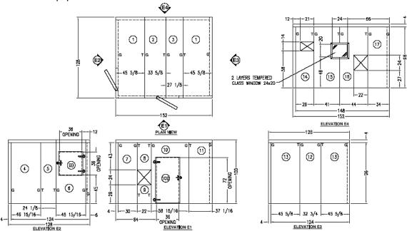
eNoise Control's solution was a modular steel acoustical enclosure. We provided cutouts for the conveyors, personnel and equipment access doors, windows to view incoming motors, air conditioning, and silenced ventilation.
