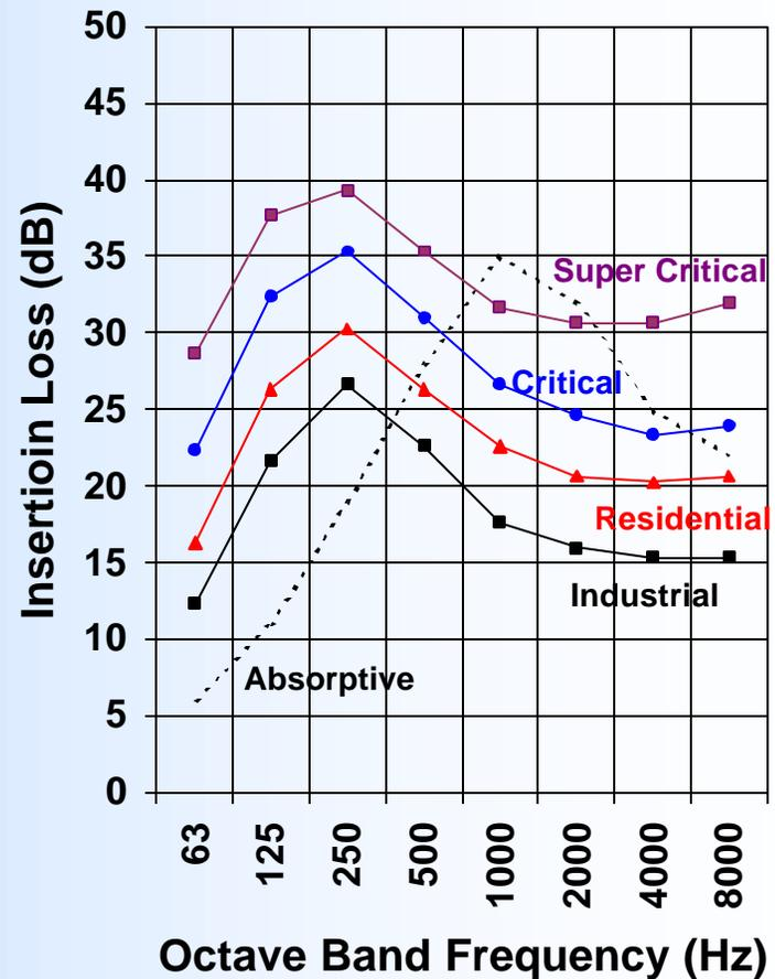
**The first step in generator exhaust noise control design is to determine if a single muffler (by itself) can meet the project requirements.**
