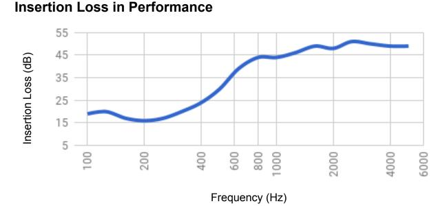
This data is representative of ASTM Test Procedure E-1222-87 for the laboratory measurement of the insertion loss of pipe lagging systems.
