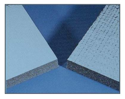
Composite foam is especially effective in dirty, greasy and damp industrial environments.
